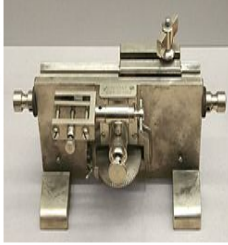
Rotary Microtome (C. Reichert, Vienna, 1905–1915)
