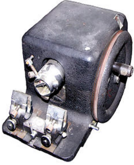
Rotary Microtome (C. Reichert, Vienna, 1905–1915)
