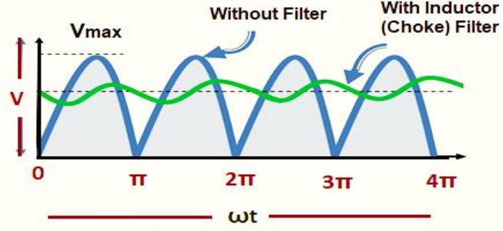
Fig:2 Series Inductor Filter Waveforms
